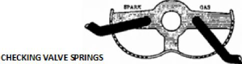
The Model T Ford service manual suggests that the valve springs be checked for strength when ever the valves are reground or replaced. This check is made by compressing the spring to 2-1/8" and the tension measured with a spring tension gauge. Yes, not every Model Towner has a spring tension gauge in their tool box.
